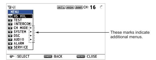
Rotate the CHANNEL/ENTER knob to select a desired menu item then push the knob. You can also select the desired menu item by pressing the 1 to 9 keys. The menu items that have a ▶ indicate additional menus.
